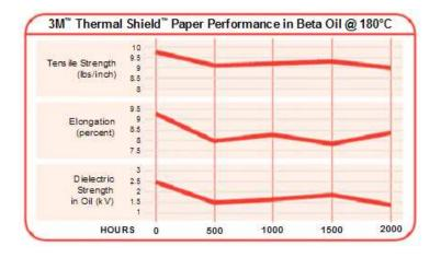
Thermal Shield Paper is compatible with oils commonly used in liquid-immersed electrical equipment and resists degradation at the elevated temperatures that may occur during overload conditions. Note that under long-term exposure in Beta oil at 180°C, 2-mil Thermal Shield Paper retains its mechanical and dielectric properties. Thermal Shield Paper displays the same high-temperature performance in mineral oil, silicone oil, and Enviro Temp FR-3.
